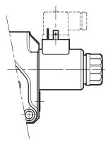
connection for DEUTSCH DT04-2P connector type code K7
