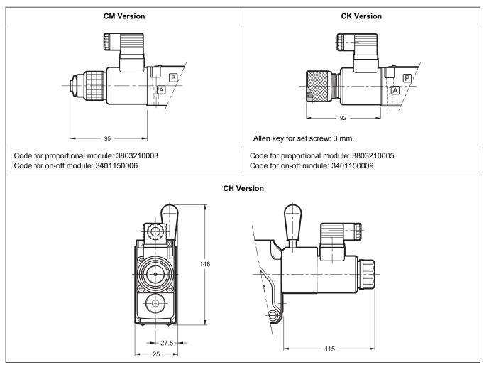
**NOTE**: The overall dimension shown in the drawings is for the proportional modules; In ON-OFF modules consider an increase of 5 mm compared to the reported dimensions.
