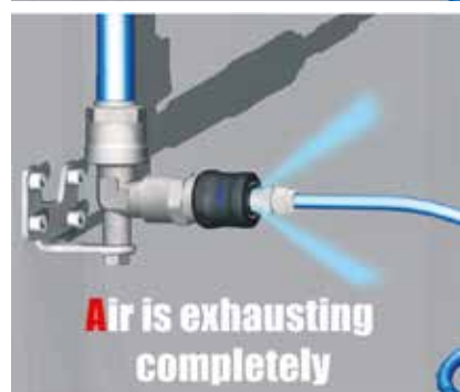
P ush the sleeve ahead and leave the hand
